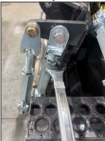
Figure 8 - Turnbuckle jam nut
