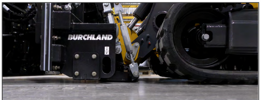
Figure 2 - Skid shoe lifts the tracks/wheels off the ground
