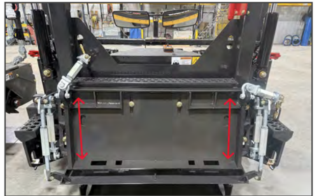
Figure 7 - Receiver plate slides up and down in slots
