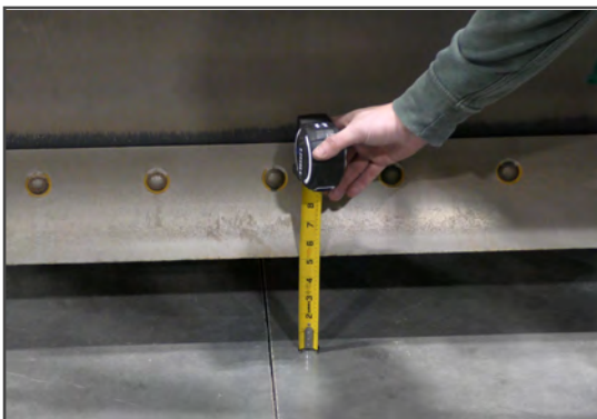
Figure 13 - Cutting edge height at 5 inches
