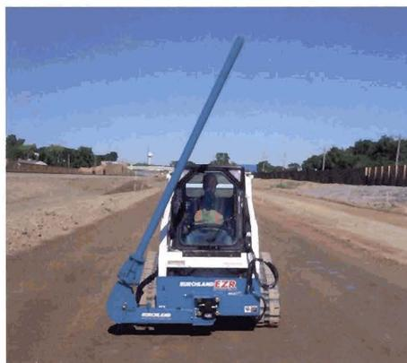
The EZR quickly and easily mounts on any skidsteer. And its Hydraulic Actuator allows the Stem to swing 180 degrees left or right, as well as angle 115° up and 8° down. Stem is detachable and available in three lengths.
