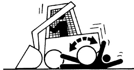
**WARNING:** Keep all people away from the machine while operating. Do not allow workers to walk near the installer while putting fabric in the ground.
