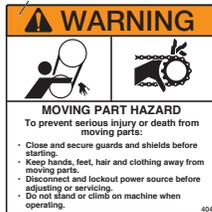
Place decal # 12081 on the bottom side of the roller chain access door.
