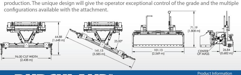
The LGX Burchland Laser Grader is proven to be a reliable attachment for finish grading. You will
