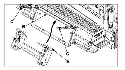
4. Raise skid steer loader arms slightly while tilting mount plate back at the same time. The trimmer should be raised and the mount plate (A) tilted far enough back to clear the ground.
